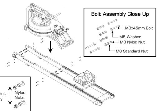
Nyloc Nuts must be outside the standard nut and Washer to properly secure assembly.
